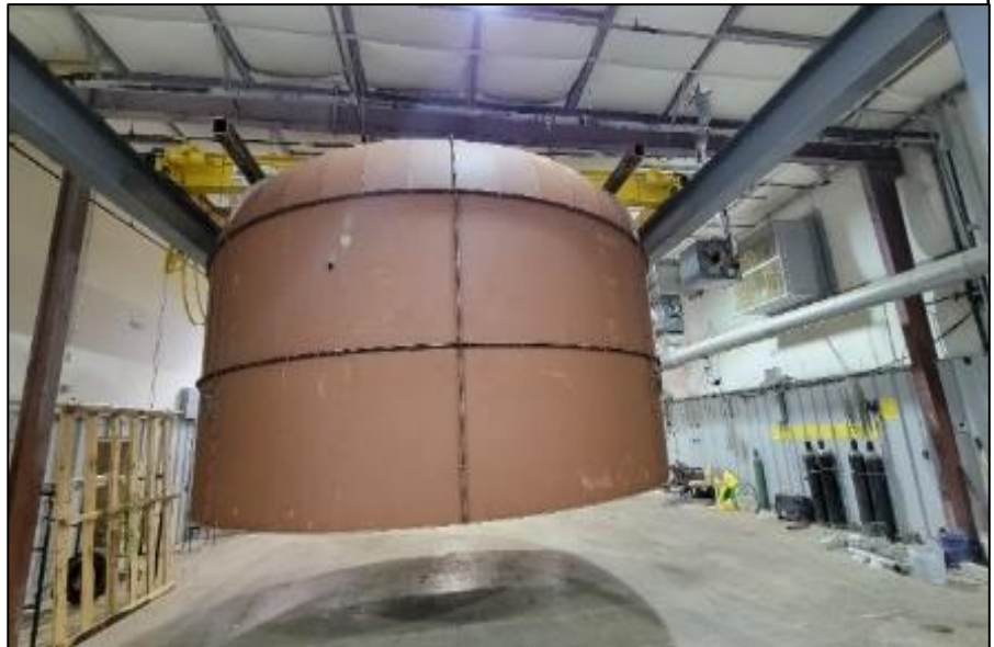
Figure 3. Sinquefeld laboratory tornado simulator at Missouri S&T
