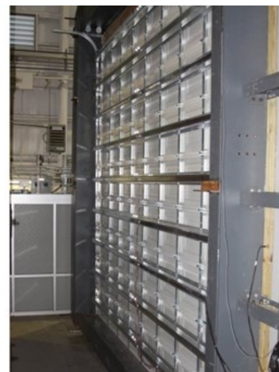
Figure 2: Sectional door 2 mounted in the pressure chamber of the simulator
