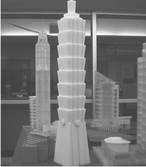
Figure 8. Tall building model tested in boundary layer wind tunnel, University of Western Ontario
