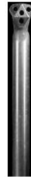
Figure 10. Dynamic multi-hole pressure probe ('cobra probe') (Picture provided by Turbulent Flow Instrumentation Pty. Ltd.)
