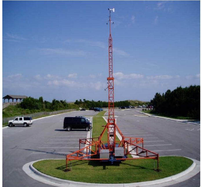
Figure 2. Tower Deployed in Atlantic Beach, NC
