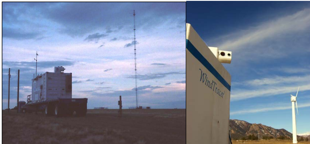
Figure 14: Mobile LIDAR systems used for wind energy measurements.
