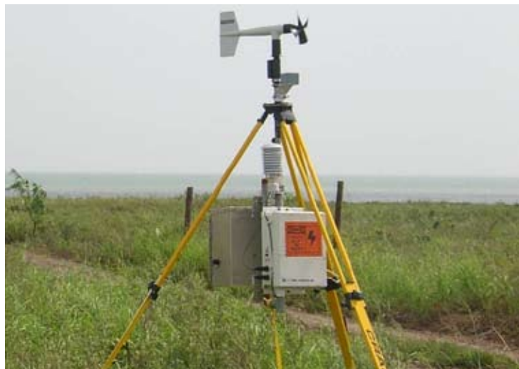
Figure 2: Stick-Net Probe deployed for Hurricane Dolly adjacent to Laguna Madre with the DAQ enclosure (white box) and the external battery enclosure (grey box) attached to the tripod.
